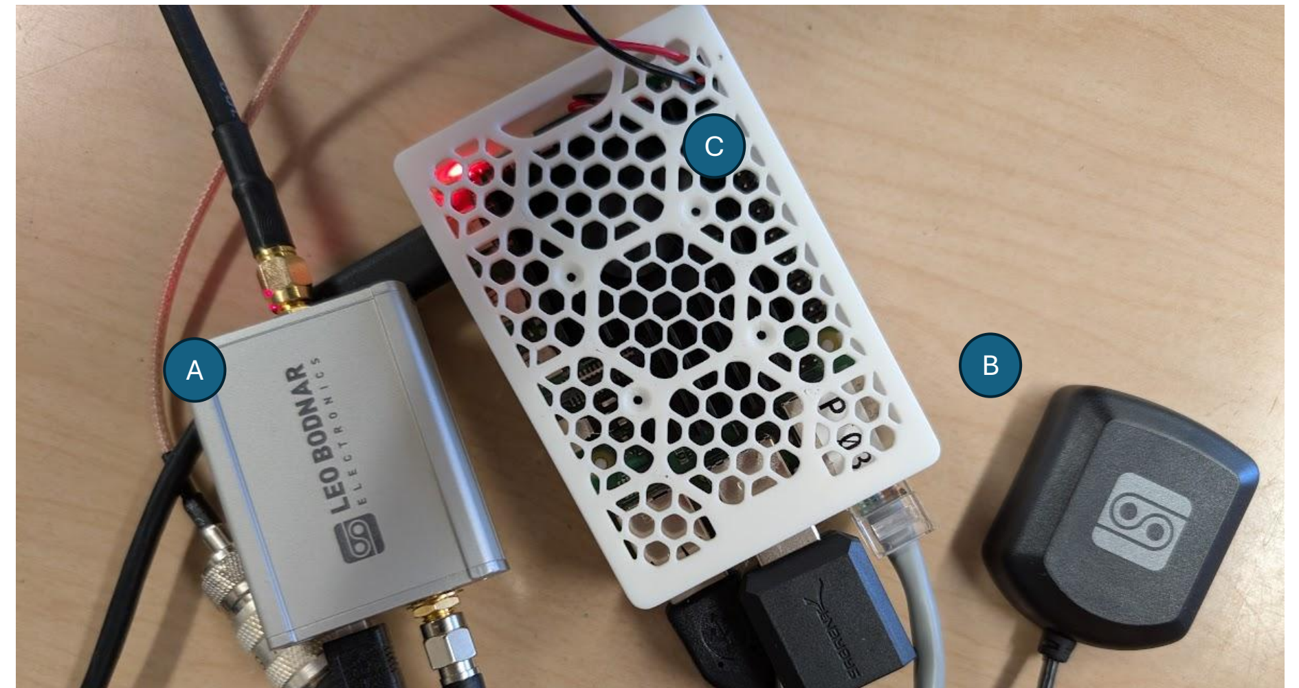
Figure 3. Grape 1 Setup. The Leo Bodnar GPSDO (A) provides a steady reference frequency at 10 MHz using a GPS antenna (B) to ensure the receiver stays on the carrier frequency. The Raspberry Pi (C) integrates the components from Figures 4 and 5 and uploads the data to the HamSCI database.
