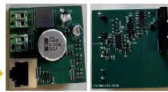
Switching Circuit Board
