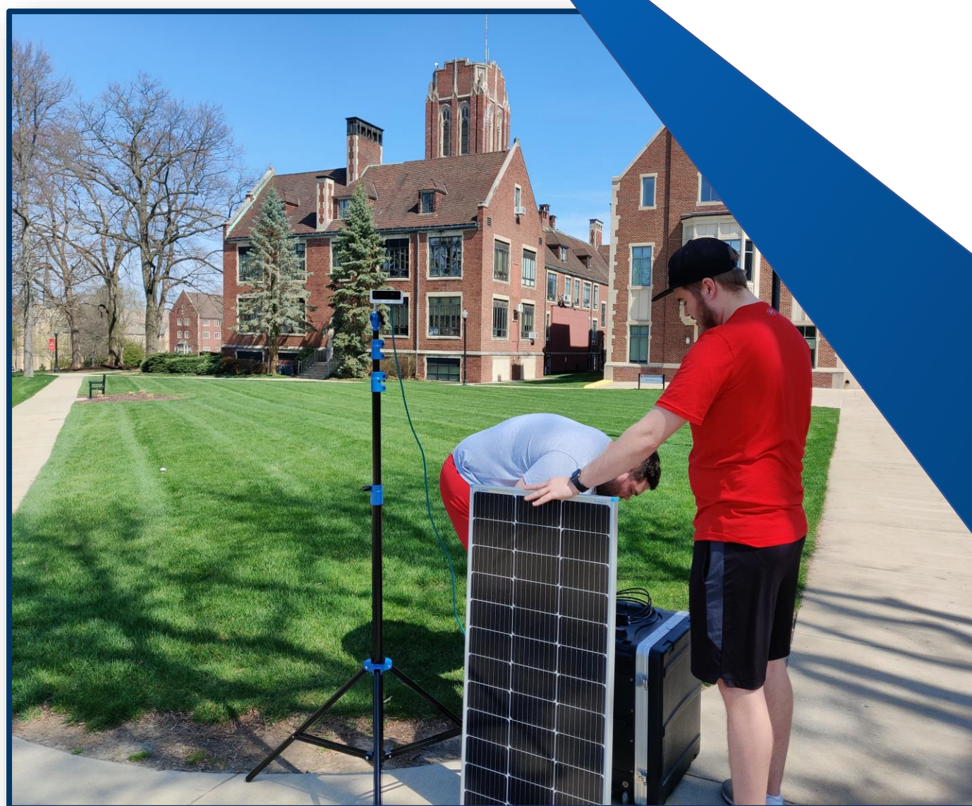
Deploying the system outside; the system is being charged through the solar panel.
