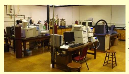
Here you can see our HPLC in the foreground, to the right our Thermal Gravimetric Analyzer and Differential Scanning Calorimeter, and on the left one of our gas chromatographs with a head-space sampler. The 300 MHZ NMR is in the background.
